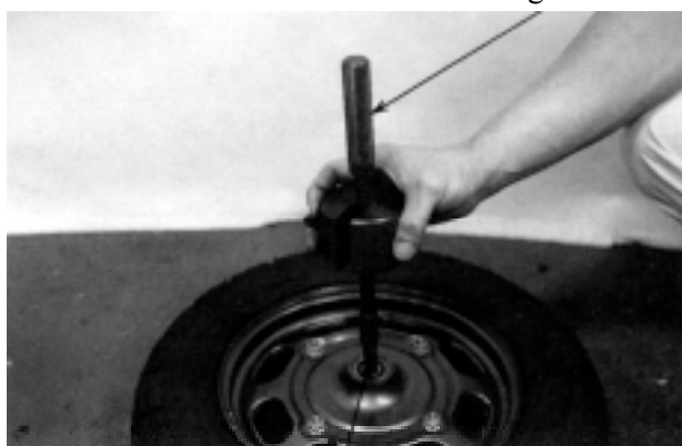
Bearing Remover Head
